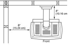
Figure 3 - Clearances for Standard Installation
